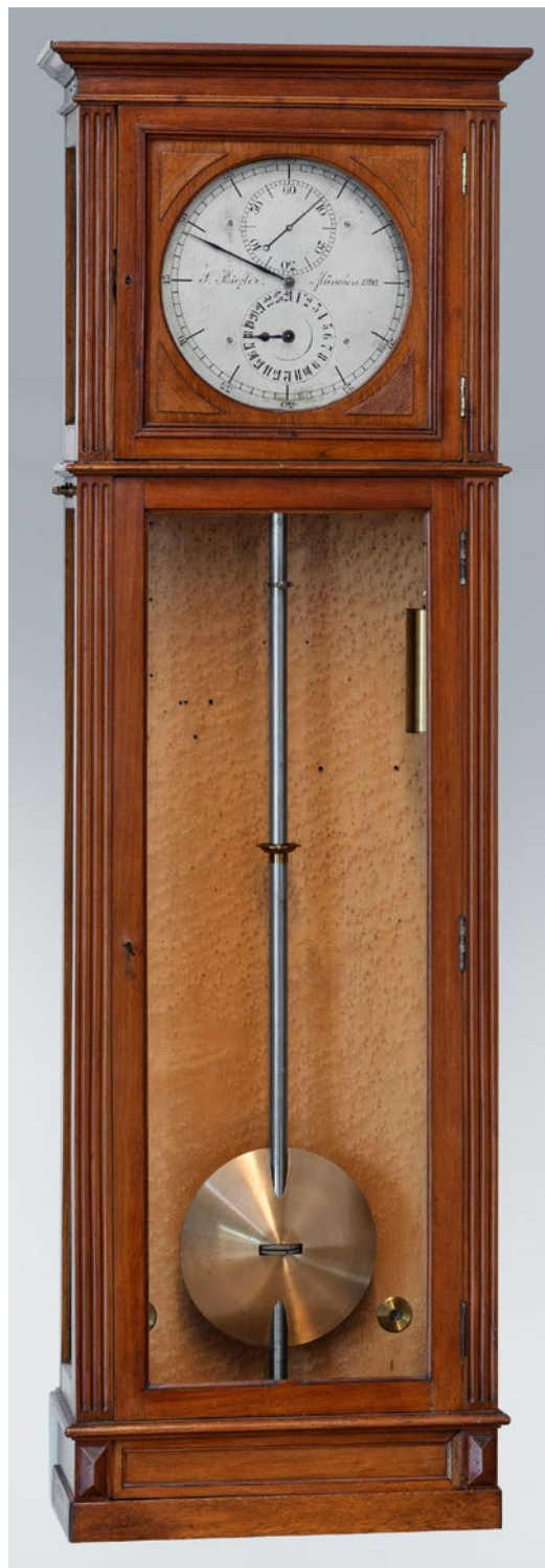
Fig. 6: Riefler clock no. 01, engraved on the dial: S. Riefler, Munich 1890. This clock was created in close collaboration with Hugo von Seeliger, then director of the Munich Observatory, and was used there from 1891 (Photo: Jürgen Ermert—Deutsches Museum München)
