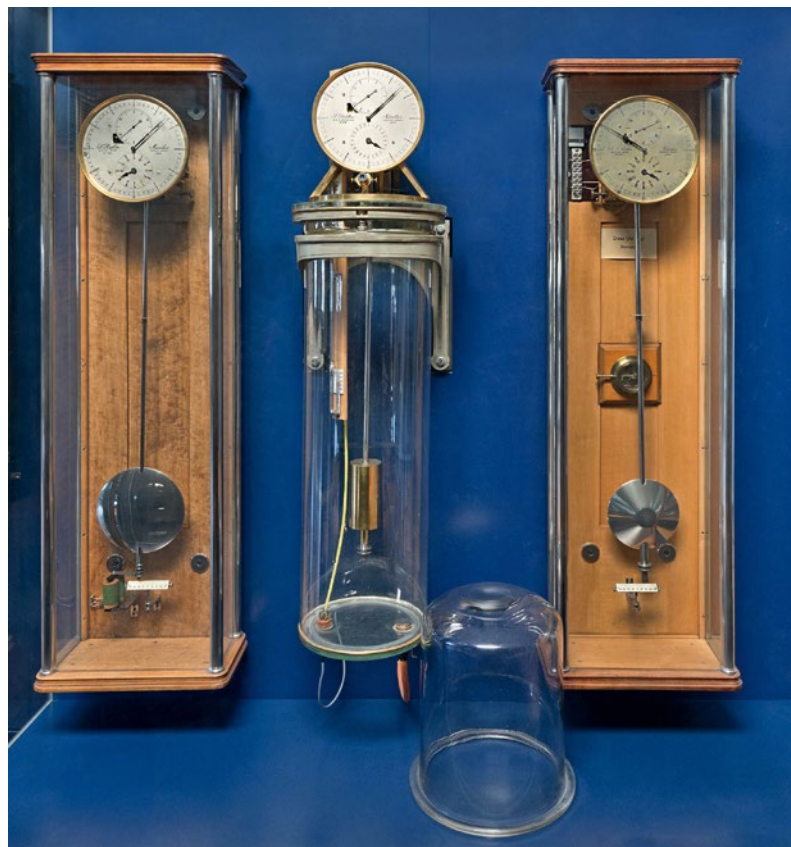
Fig. 12: Time-keeping system in the Deutsches Museum with master clock no. 98 in the glass tank and two slave clocks (Photo: Jürgen Ermert.-Deutsches Museum)
