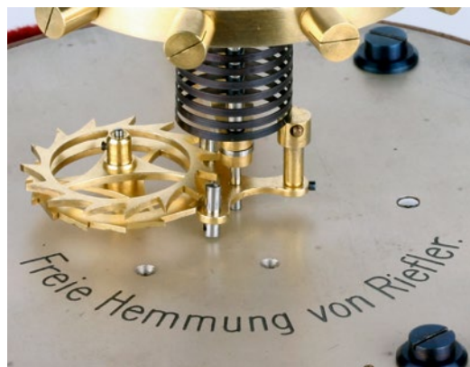
Fig. 3: Model for new escapement with a completely freely oscillating balance and driven via the balance spring stud (Photo: Dieter Riefler)
